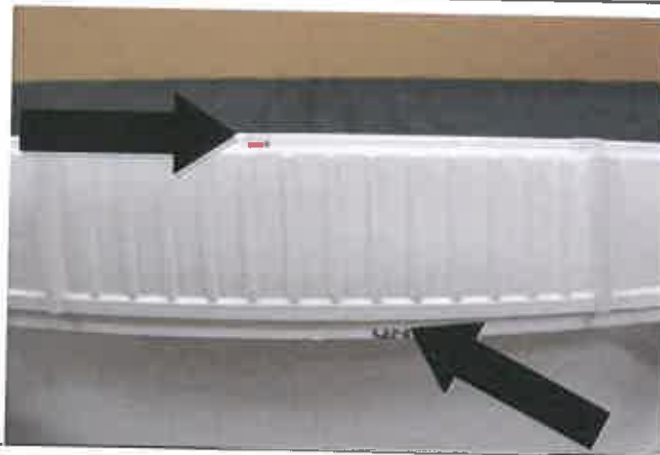
Illustration 5- Example of lid fully tightened, gasketed pail, window to left of UN mark.
