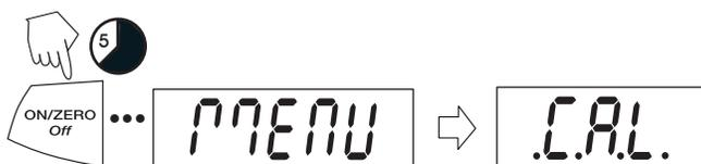
3. Press and release **ON/ZERO Off**. Scale will flash **-C-** and show required weight. Place the calibration weight on the scale.
