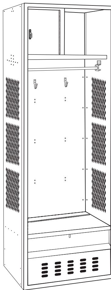
16. Bolt one coat rod bracket (14) to one of the sides (2). Then, insert coat rod (13) into the coat rod bracket (14) that is bolted to the side (2). Place second coat rod bracket (14) over the other end of the coat rod (13). Bolt second coat rod bracket (14) to the other side (2). (See Figure 14)
