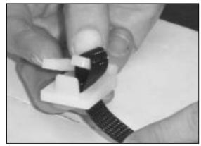
Insert end of strapping up through center of the buckle and around open leg to form a loop. Pull top tight around leg.
