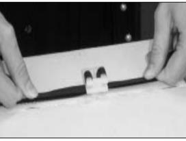
Pull both top ends of strapping in the opposite direction to manually tighten.
