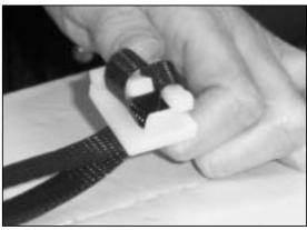
Wrap strapping around package. Loop strapping around remaining open leg of buckle. Pull loop tight around leg.
