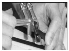
Use blade side of tool. Cut away excess strapping.
